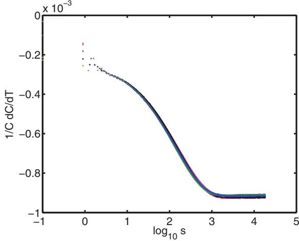
FIG. 6. (Color) The relative change in  $C$  divided by the size of the temperature step. The data shown are the same data as in Fig. 5, and the colors used for each curve are the same. All the curves superpose, which demonstrates that the experiment is linear. Moreover, it demonstrates that the subtraction of the background drift is successful.
