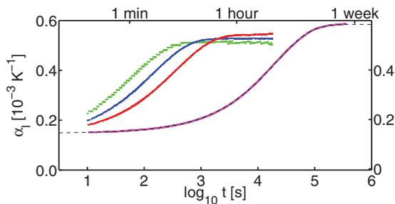
FIG. 7. (Color) The measured time-dependent expansion coefficient of tetramethyl tetraphenyl trisiloxane at  $T = 205, 209, 210,$  and  $211$  K. At the lowest temperature we also show a fit to the modified stretched exponential Eq. (15).
