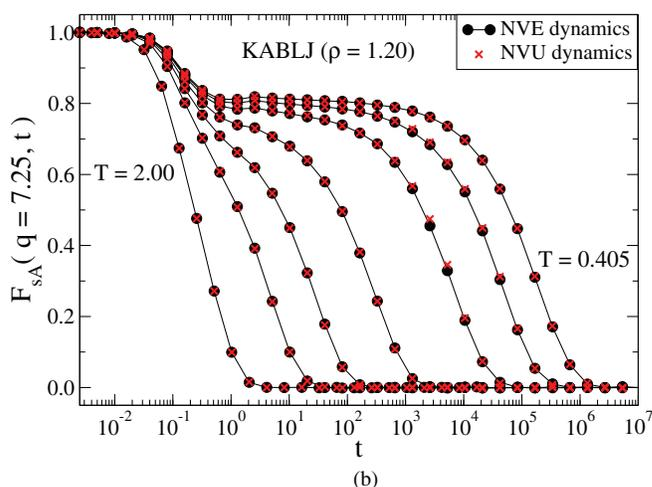
FIG. 3. (a) Mean-square displacement and (b) incoherent intermediate scattering function at the wave vector of the first peak of the AA structure factor. Both simulations were performed at  $\rho = 1.2$  for  $T = 2.0, 0.80, 0.60, 0.50, 0.44, 0.42$ , and  $0.405$  (left to right) for the KABLJ liquid (1024 particles). *NVE* dynamics is given by the filled black circles connected by straight lines, *NVU* dynamics by the red crosses.
