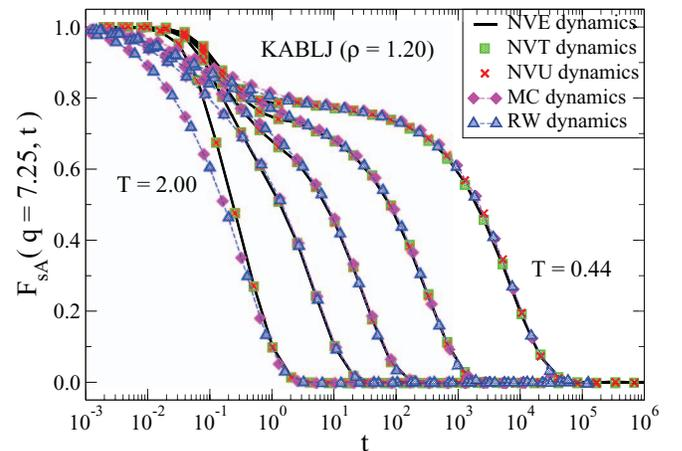
FIG. 7. The incoherent intermediate scattering function for all five investigated dynamics for the KABLJ liquid at  $\rho = 1.2$  and  $T = 2.0, 0.80, 0.60, 0.50$ , and  $0.44$ . The black curve is the  $NVE$  simulation, red crosses:  $NVU$ , green squares:  $NVT$ , magenta diamonds:  $MC$ , blue triangles:  $RW$ .
