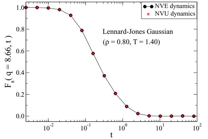
FIG. 5. The incoherent intermediate scattering function at  $\rho = 0.8$  and  $T = 1.4$  for the Lennard-Jones Gaussian system.<sup>18</sup> The black circles represent a *NVE* simulation, the red symbols represent a *NVU* simulation.
