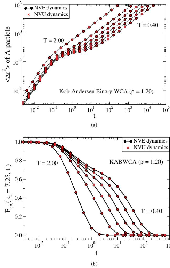
FIG. 4. (a) Mean-square displacement and (b) incoherent intermediate scattering function at the same wave vector as in Fig. 3. Both simulations were performed at  $\rho = 1.2$  for  $T = 2.0, 0.80, 0.60, 0.50, 0.44$ , and  $0.40$  (left to right) for the WCA approximation to the KABLJ liquid. *NVE* dynamics is given by the filled black circles connected by straight lines, *NVU* dynamics by the red crosses.
