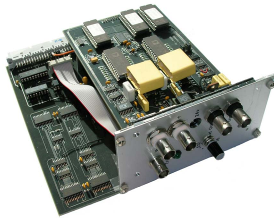
FIG. 8. (Color online) Circuit boards containing components for the custom-built frequency generator.
